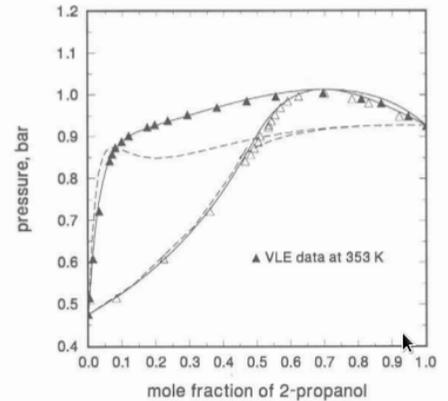
Figure 3.5.3. VLE correlation of the 2-propanol and water binary system at 353 K with the 2PDWW mixing rule and the PRSV equation of state. Solid lines denote correlation results with  $k_{12}/k_{21} = 0.0953/0.0249$ . Dashed lines show 1PDWW model correlations presented earlier in Figure 3.4.5. (Points are the data of Wu et al., 1988; data file for this system on the accompanying disk is 2PW80.DAT.)
